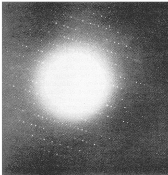
Electron diffraction pattern of a catalase crystal which was frozen in liquid nitrogen
