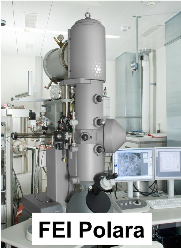
Microscope cooled internally
